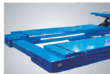
Optional LED lighting: 24V protected LED light Bar.
