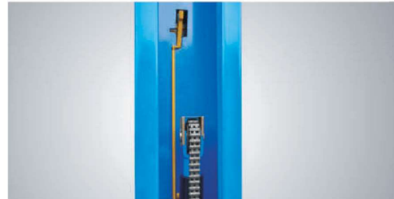
▲ Dual safety device, with chain protection cover to prevent it take off.
