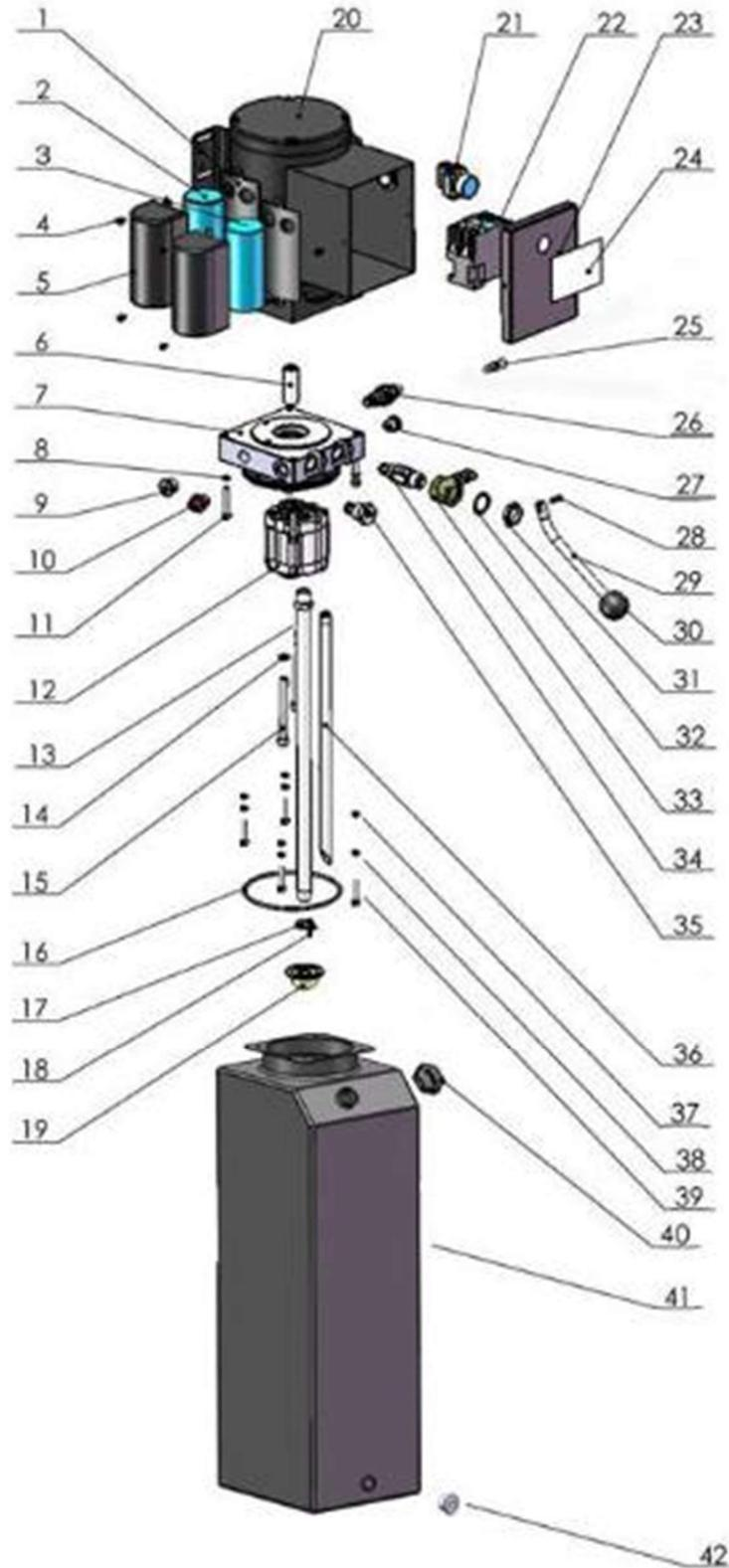
**Fig.51** 220V/60Hz Single Phase Manual Power Unit Exploded View
