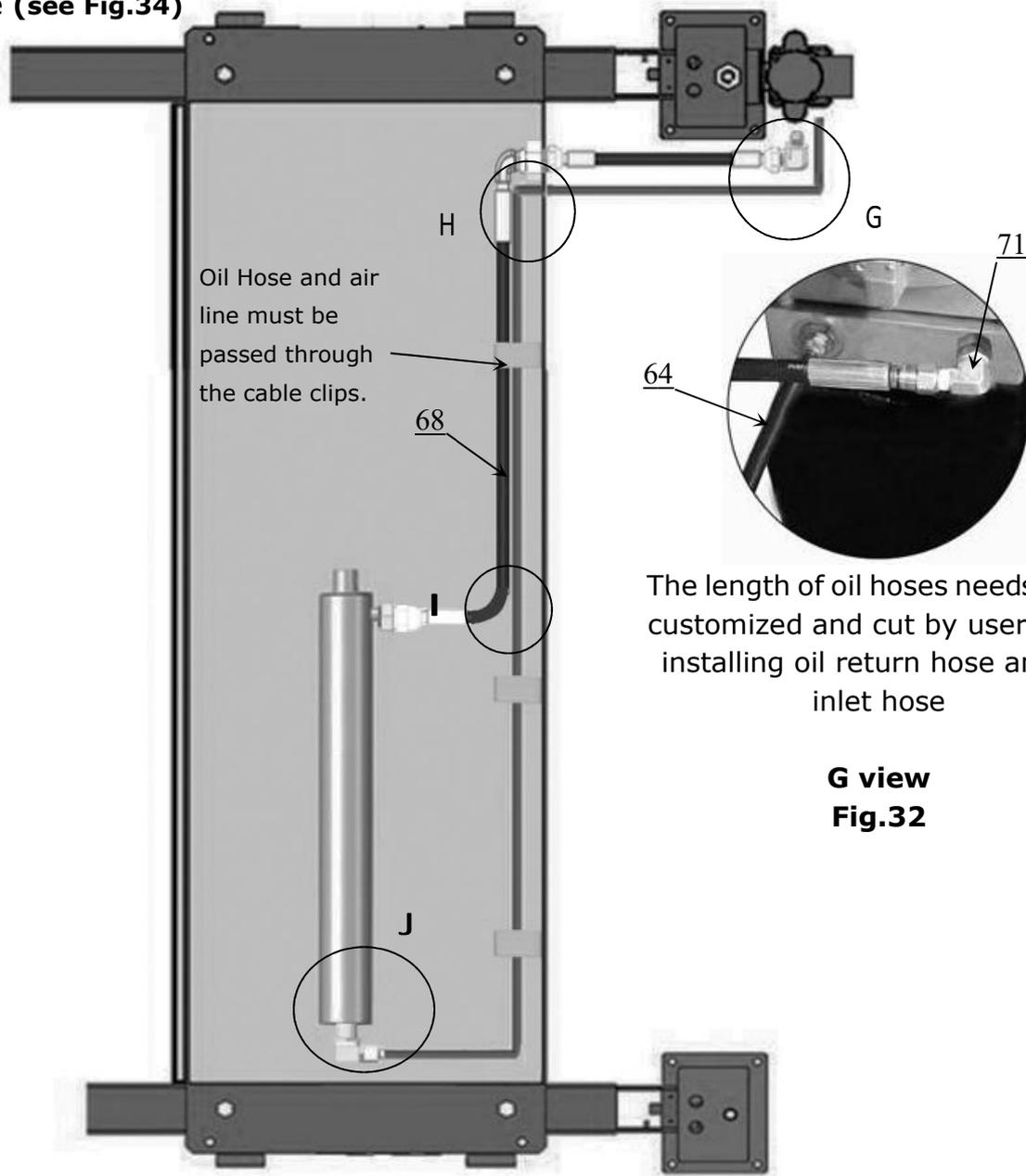
The length of oil hoses needs to be customized and cut by user when installing oil return hose and oil inlet hose
