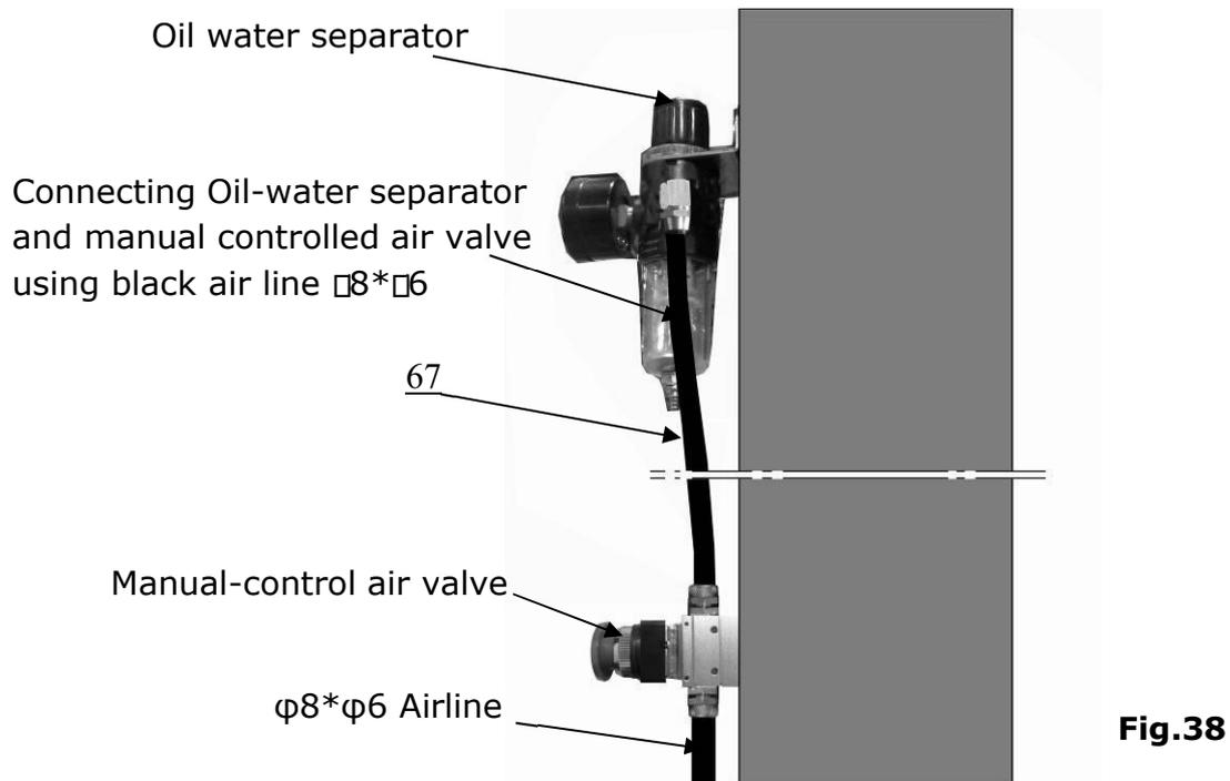
5. Connecting air inlet (Air supply pressure 8 kg/cm<sup>2</sup>), adjusting the air pressure of Oil-water separator to 0.8 MPa (**See Fig.39**)
